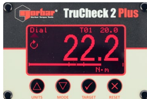
TruCheck™ 2 Plus display showing above target tolerance
