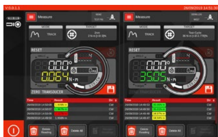
Displaying 2 transducer readings simultaneously
