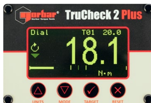
TruCheck™ 2 Plus display showing below target tolerance
