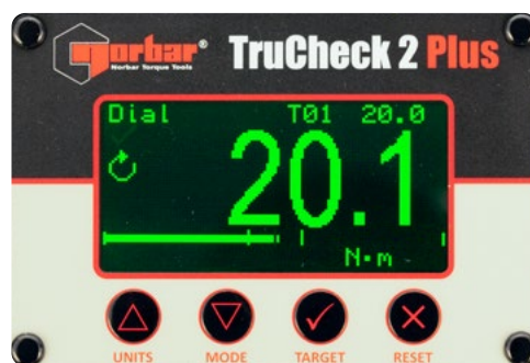
TruCheck™ 2 Plus display showing within target tolerance
