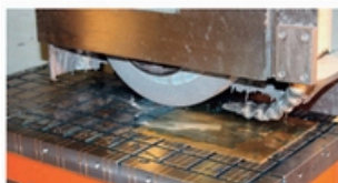
An example of grinding of brass by utilizing the permanent electromagnetic feature
