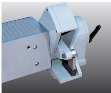
Gauge block setting location on the right side (photo): R type, and on the left side: L type.
