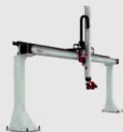
gantryRobot as multi-axial portal robot
