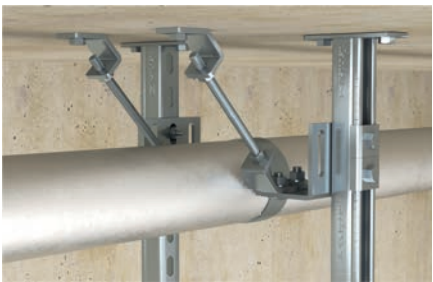
Longitudinal pipe bracing with FTRB 45
