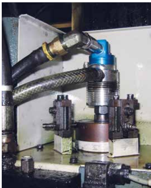
DEUBLIN 1109 on vertical machining center
