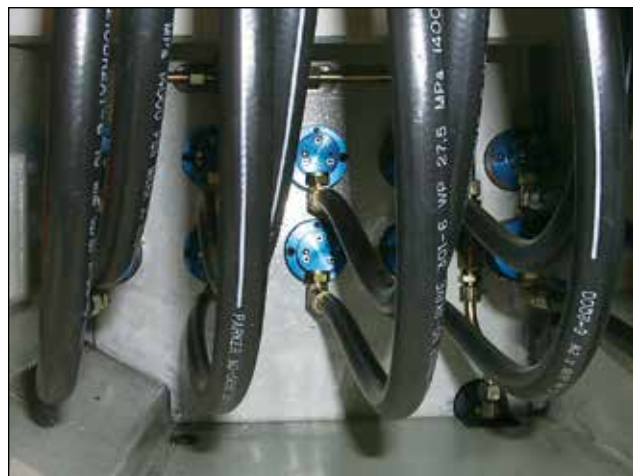
DEUBLIN 1117 Bearingless Unions on Automotive Transfer Line
