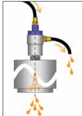
Tool change with vertical spindle
