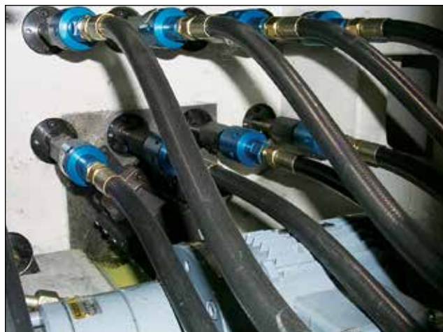
DEUBLIN 1116 Bearing-Supported Unions on Automotive Transfer Line
