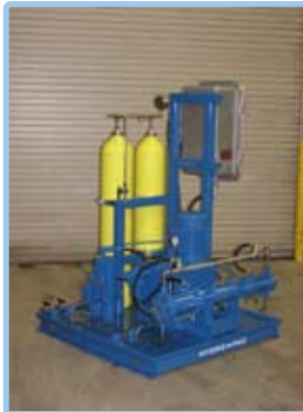
Five horsepower compressor packaged with gas storage cylinders.
